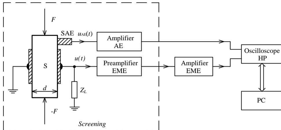
**Figure 1:** Initial set-up for experimental measurement
