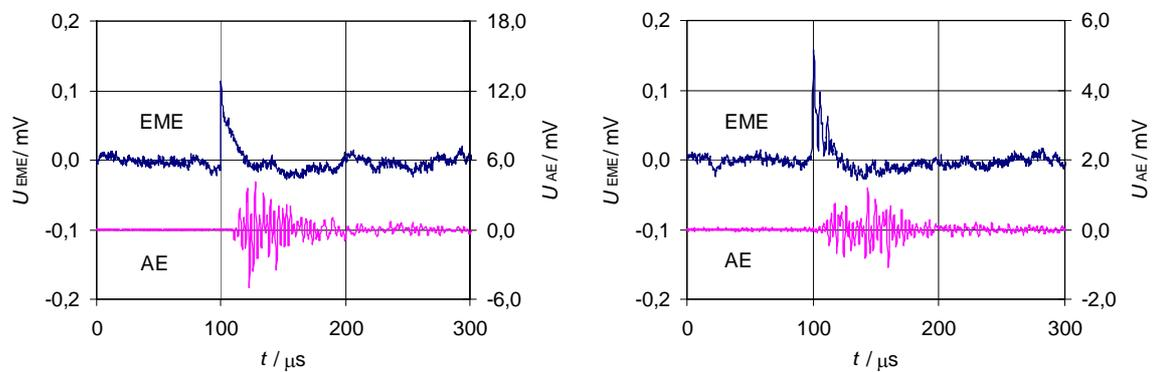
**Figure 2:** Typical EME and AE time behavior examples
